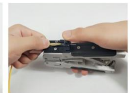
⑤: Strip the 0.9 fiber sheath
