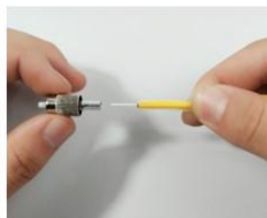
⑦: Thread the fiber through the ferrule
