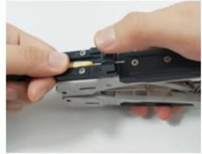
⑤: Strip the 0.9 fiber sheath
