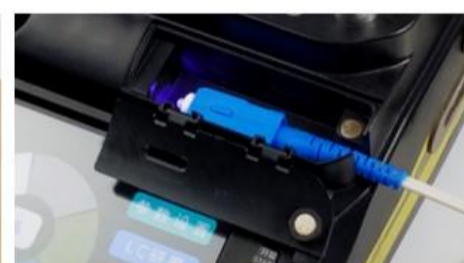
⑧: Install the sleeve of tail handle and solidify inside the machine
