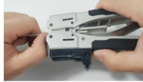
④: Strip the determined length
