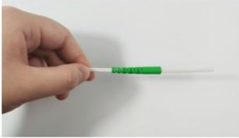
②: Thread the sleeve of tail handle
