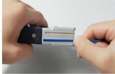
③: Determine the fiber length
