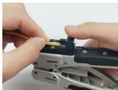
⑥: Strip the fiber coating
