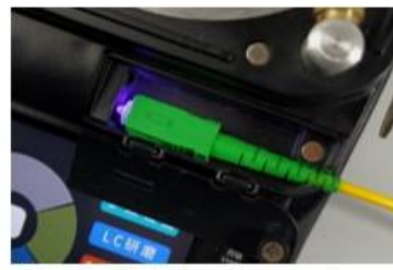
⑨: Install the sleeve of tail handle and solidify inside the machine
