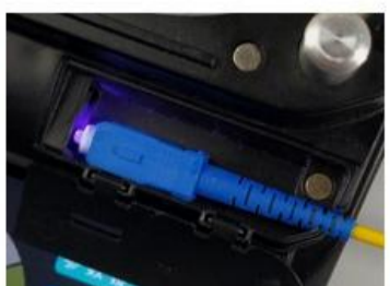
⑨: Install the sleeve of tail handle and solidify inside the machine
