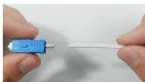
⑥: Thread the fiber through the ferrule
