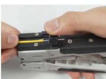
⑤: Strip the 0.9 fiber sheath
