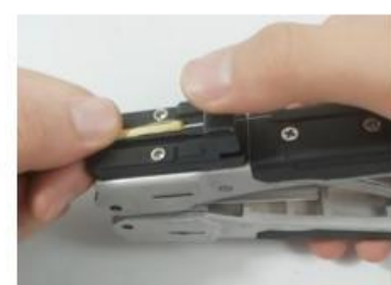
⑥: Strip the fiber coating
