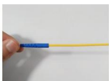
②: Thread the sleeve of tail handle
