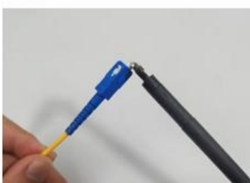
⑩: Use a cutter to remove excess fiber and start polishing
