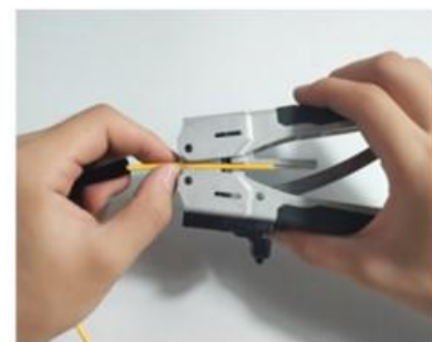
③: Strip according to the determined length
