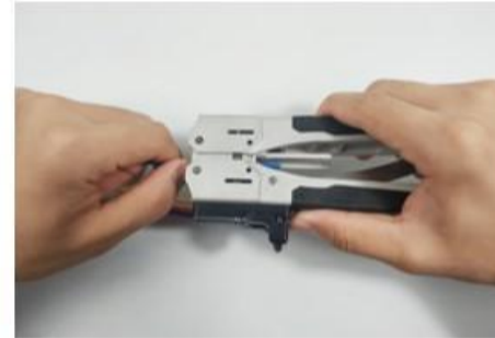
④: Strip the determined length
