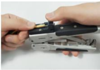
⑥: Strip the fiber coating
