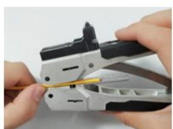
③: Strip according to the determined length
