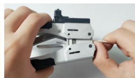
④: Strip according to the determined length
