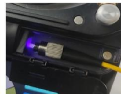
⑨: Install the sleeve of tail handle and solidify inside the machine
