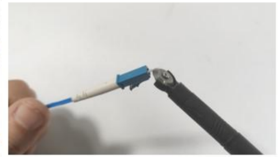
⑨: Use a cutter to remove excess fiber and start polishing
